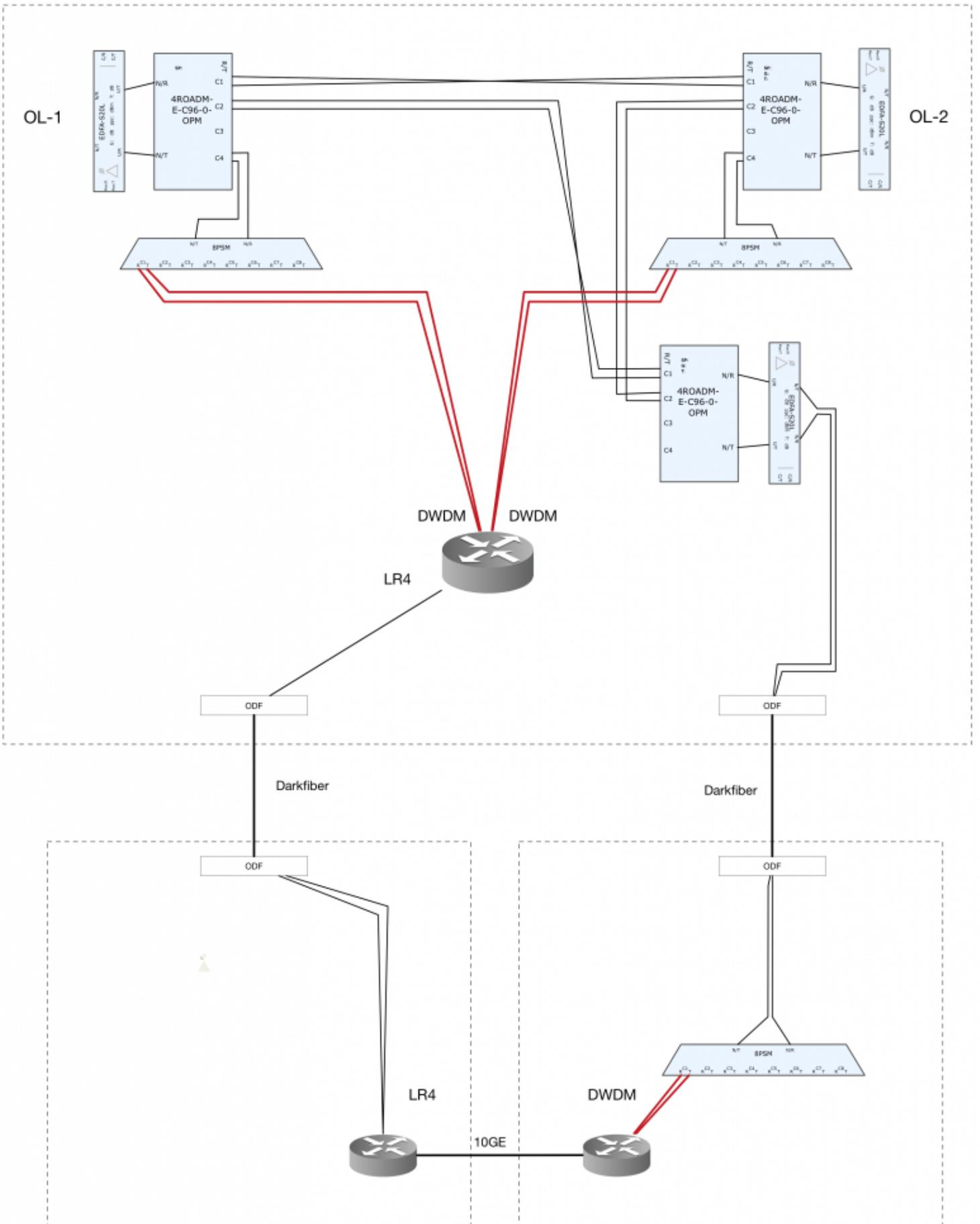
This is a more block-diagram how it will look on how it will be connected if its a Standard type of handoff. Click it for the full resolution to see how the idea is to connect things. The 8PSM "filter" is a passive splitter/combiner and is gridless.
