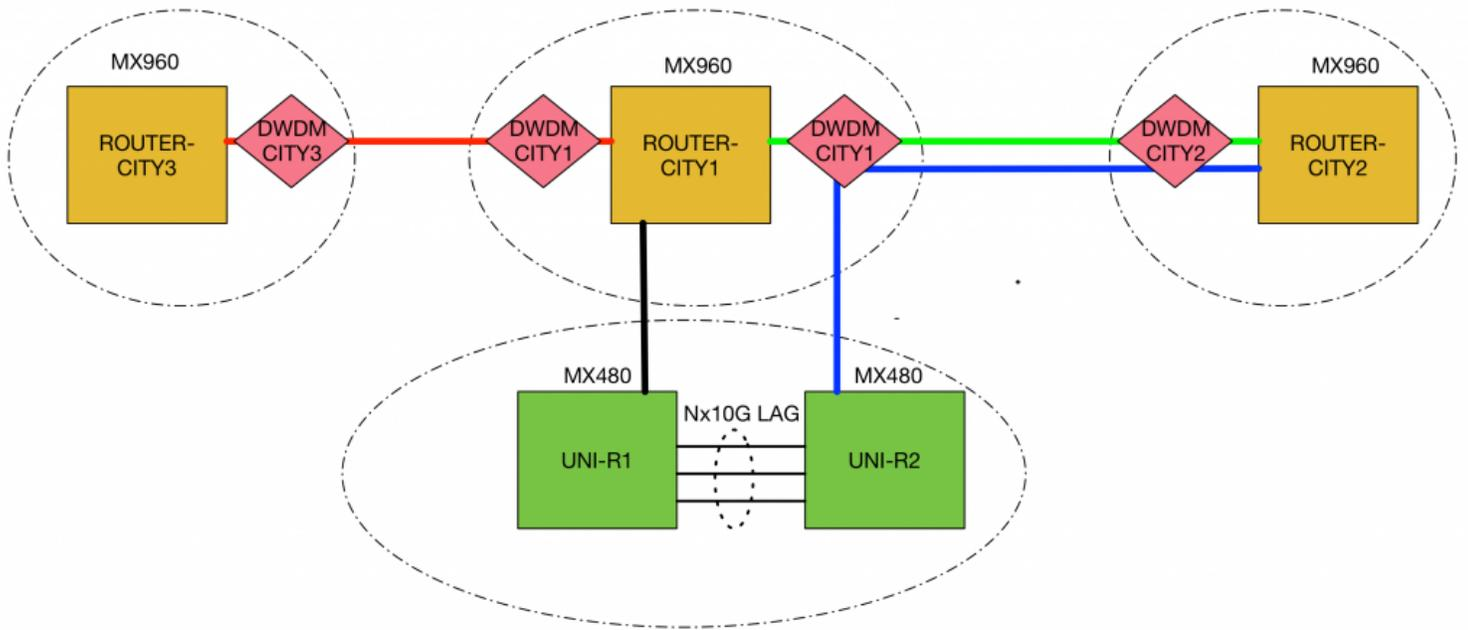
This is a very simple overview on the physical design of university-access. There is two Juniper MX480 located on a diverse location at campus, these are tied together with fiber in between consisting of Nx10G. The uplinks is one 100G LR4 locally in the city, and a 100G Coherent to the neighbouring city. And then the core-router in the city is also tied together to two neighbouring cities using 100G Coherent interfaces.
