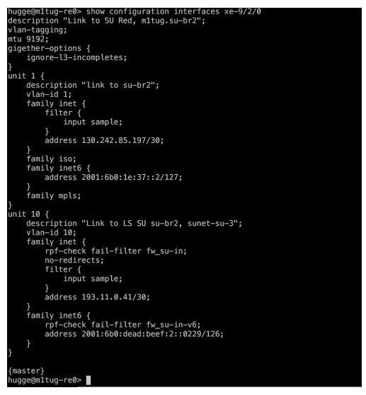
So this is configuration for "Stockholms Universitet" from old Optosunet (it will look the same in Sunet-C). Vlan 10 here is the uplink towards SU (the other is our vlan for our logical system) so it's directly facing SU and is also the VLAN we run the BGP-peering in. Here we can see rpf-checks being configured with a fail-filter "fw\_su-in"
