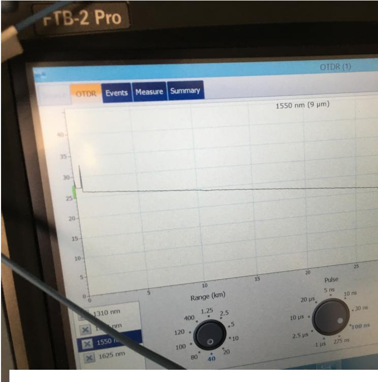
OTDR measurement on one fiber of the pair going northbound, distance is as expected an
